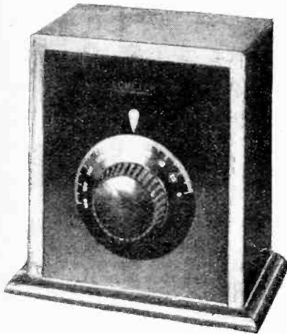
The Lometer, an absorption wavemeter covering wavelengths from 22 to 70 metres.
